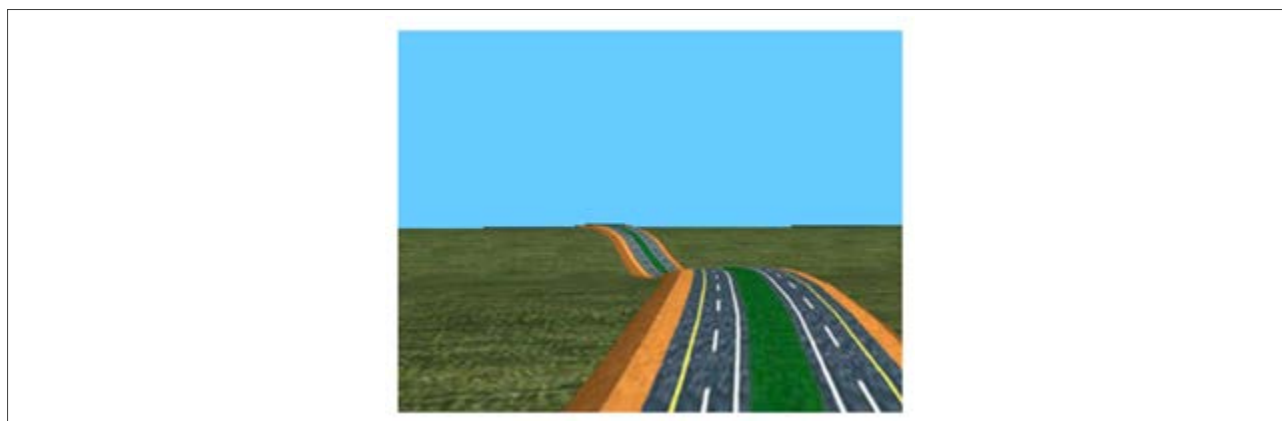
Figure 7.7 Variable Gradients (Rolling Grade-line)
