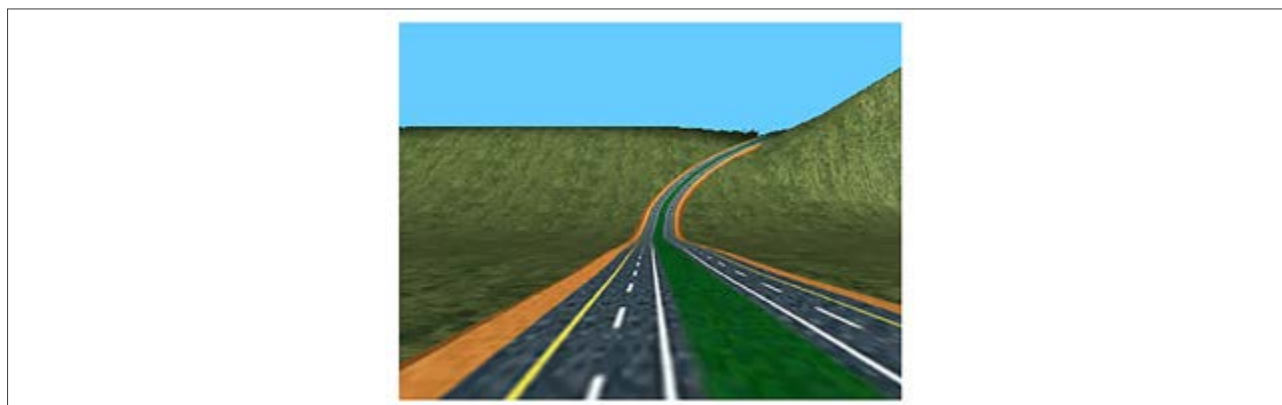
Figure 7.3 Out-of-phase Vertical and Horizontal Alignments
